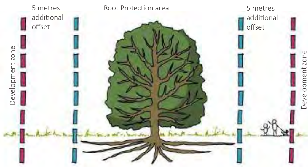
Typical section of root protection area including additional 5 metre offset
